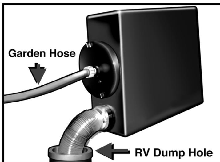
Disconnect water supply hose. Remove 6" cap and look to see if tank is thoroughly clean. Repeat cleaning process if necessary.
